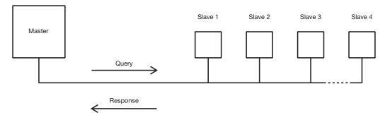
In the MODBUS Protocol the master can address individual slaves, or, using a special "Broadcast" address, can initiate a broadcast message to all slaves. The MPA-1 does not support the broadcast address.
