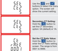
The CT Rate is the CT Primary divided by the CT Secondary. For Example: 200/5A Current Transformers - 200÷5=40, so the CT Rate would be 0040 and the CT2 would be 5.
