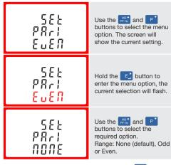
On completion of the entry procedure, hold the E button for 3 seconds until the selection stops flashing
