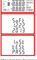
The first screen lights up all display segments and can be used as a display check.
