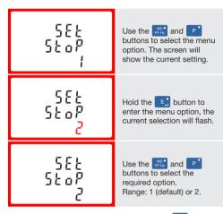
On completion of the entry procedure, hold the statement button for 3 seconds until the selection stops flashing
