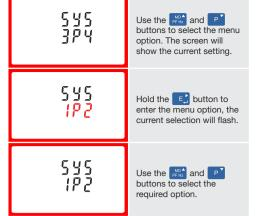
Hold the button to confirm your adjustment. Hold the button for 3 seconds to exit the set up menu.
