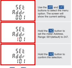
Use the press the buttons to choose the necessary number, then press the button to move along to the next number. To save the new setting, hold the button for 3 seconds until the selection stops flashing
