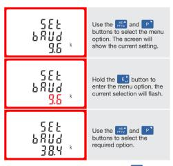
On completion of the entry procedure, hold the button to confirm the setting.
