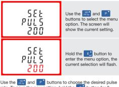
Use the prize and buttons to choose the desired pulse rate. To save the new setting, hold the button for 3 seconds until the selection stops flashing.
