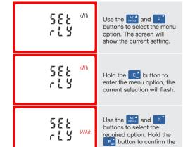
Hold the MA button for 3 seconds to exit the set up menu.
