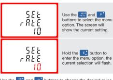
Use the property and p buttons to choose the desired pulse rate. To save the new setting, hold the button for 3 seconds until the selection stops flashing
