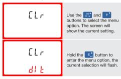
Hold the button to confirm the setting and press Ma to return to the main set up menu.
