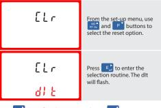
Press E to confirm the setting and press WA to return to
