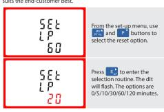
Press to confirm the setting and press what to return to the main set up menu.
