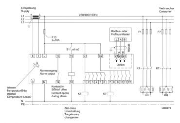
Diagr.: Connection example, power factor controller with measurement and supply voltage L-N,12 relais outputs, target cos(phi) changeover and alarm output.
