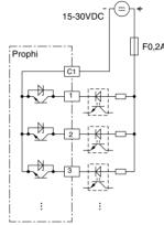
Diagr.: Connection example "Transistor outputs"
