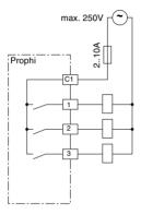
Diagr.: Connection example "Relay outputs"
