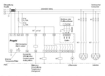
Diagr.: Connection example, power factor controller with measurement and supply voltage L2-L3,12 relais outputs, target cos(phi) changeover and alarm output.
