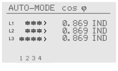
Example 2: Automatic operation (Mixed Mode) L1...L3: phase wise compensation by single phase capacitors
