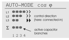
Example 3: Automatic operation Measuring in one phase Controlling of 15 three-phase-capacitors
