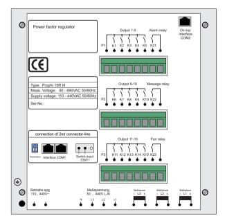
The allocation of switching outputs K1...K15 to the capacitors complies to the selected connection variant and the desired CONTROL-MODE (Programming/point 2)
