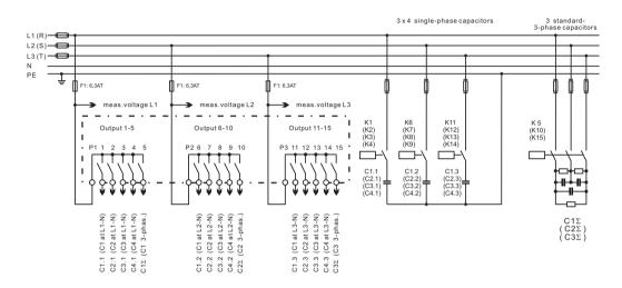
In case of the setting the controller will automatically assign the capacitors according to the wiring diagram.
