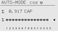
Number of switching outputs until end stop. Here: 15 three-phase capacitors, end-stop: 15 Control direction is symbolized by a compact arrow: Connecting-in
