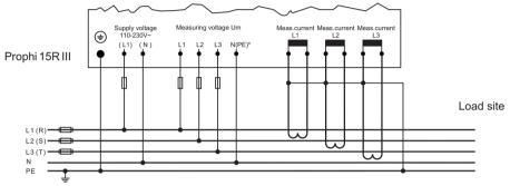
Alternative 2: single-phase measuring via current transformer in L1 Values extrapolated (balance assumed). Measuring complies with conventional measuring for switching of three-phase capacitors. Use: CONTROL-MODE 5
