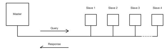
In the MODBUS Protocol the master can address individual slaves, or, using a special "Broadcast" address, can initiate a broadcast message to all slaves. The MPA-3 does not support the broadcast address.
